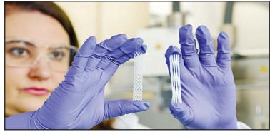
Nicole Black, Ph.D., VP of Biomaterials and Innovation at Desktop Health, examines two tubular medical devices printed on the new 3D-Bioplotter® PrintRoll™ rotating build platform in medical-grade materials. sizes. Rotating speed is tightly controlled by the 3D-Bioplotter's easy-touse software.
