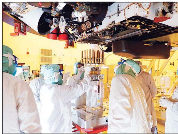
In this May 20, 2020 photo, made available by NASA/JPL-Caltech, engineers and technicians insert sample tubes into the belly of the Perseverance Mars rover at the Kennedy Space Center in Florida. (AP)
