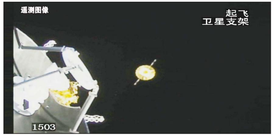
This photo taken by satellite bracket camera of Long March-8 carrier rocket on March 20, 2024 shows the Queqiao-2 relay satellite (center) successfully separating from the carrier rocket with its solar wing and antenna successfully unfolded. (Xinhua)
