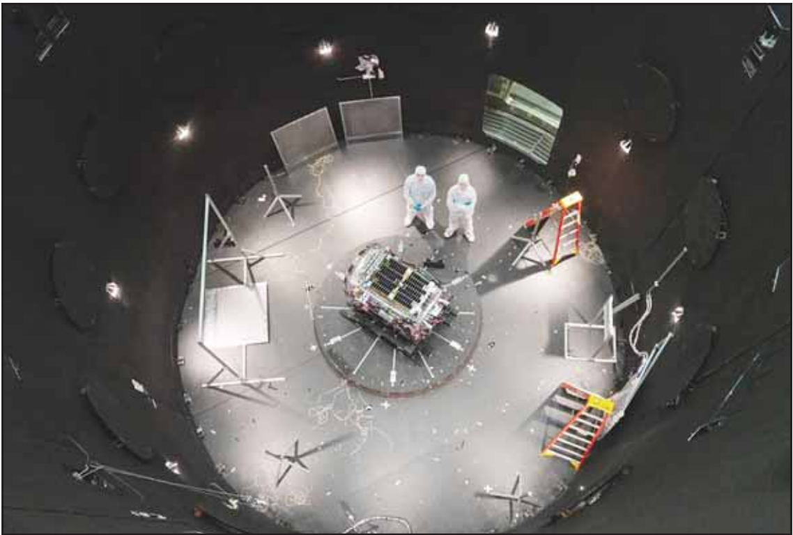
This photo provided by NASA shows Kieran Wilson, LINK’s principal investigator, and Hunter Robertson, a space systems engineer, both at Katalyst Space, standing next to their spacecraft inside the SES (Space Environment Simulator) at NASA’s Goddard Space Flight Center in Greenbelt, Md. on April 17, ahead of thermal vacuum testing. (AP)
