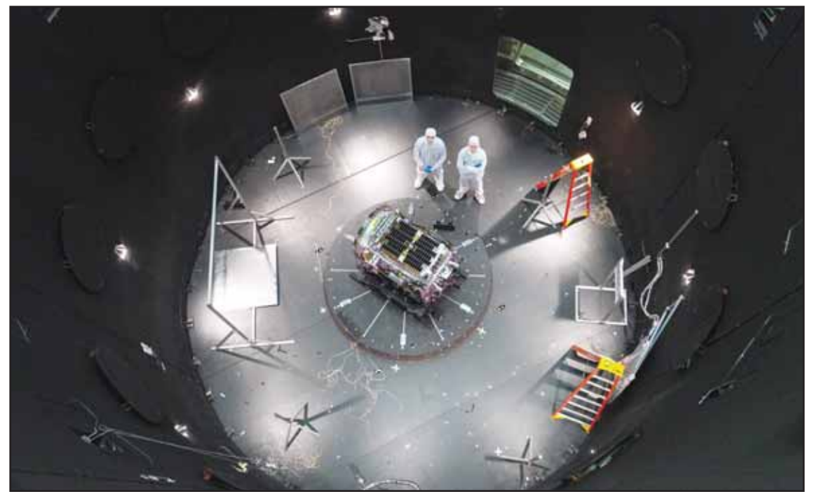
This photo provided by NASA shows Kieran Wilson, LINK's principal investigator, and Hunter Robertson, a space systems engineer, both at Katalyst Space, standing next to their spacecraft inside the SES (Space Environment Simulator) at NASA's Goddard Space Flight Center in Greenbelt, Md., April 17, 2026, ahead of thermal vacuum testing. (AP)
