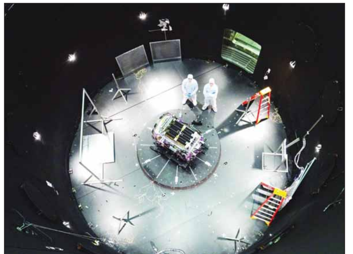
This photo provided by NASA shows Kieran Wilson, LINK's principal investigator, and Hunter Robertson, a space systems engineer, both at Katalyst Space, standing next to their spacecraft inside the SES (Space Environment Simulator) at NASA's Goddard Space Flight Center in Greenbelt, Md on April 17, ahead of thermal vacuum testing. (AP)
