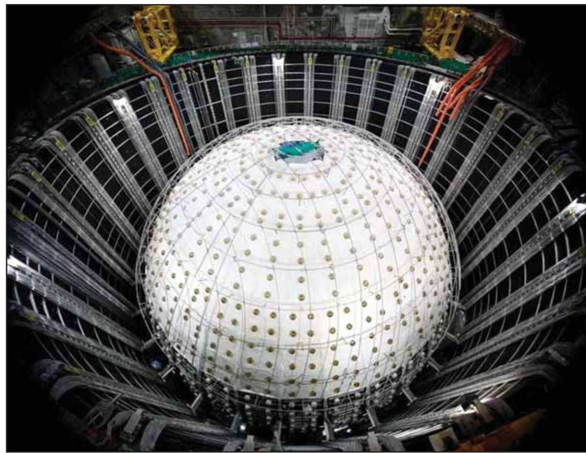
This stitched photo taken on Oct 9, 2024 shows the central detector of the Jiangmen Underground Neutrino Observatory (JUNO) in Jiangmen, south China's Guangdong Province. (Xinhua)
