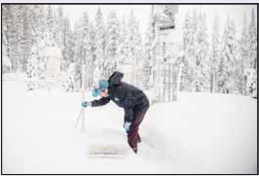
Dr Gabe Lewis, a research scientist, measures snow depth and mass to calculate density and snow water equivalent at Central Sierra Snow Lab in Soda Springs, Calif on Jan 5. (AP)
