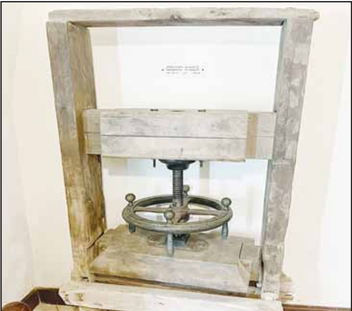
A manual wooden printing press whose primary function was to press the paper onto the inked die to transfer the printed letters.
