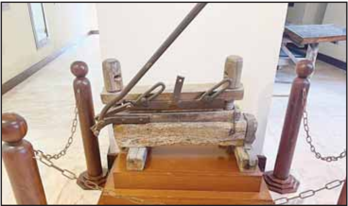
Manual printing scissors, or what is known as an old paper-cutting machine, was used in the Al-Zakhriya printing press.
