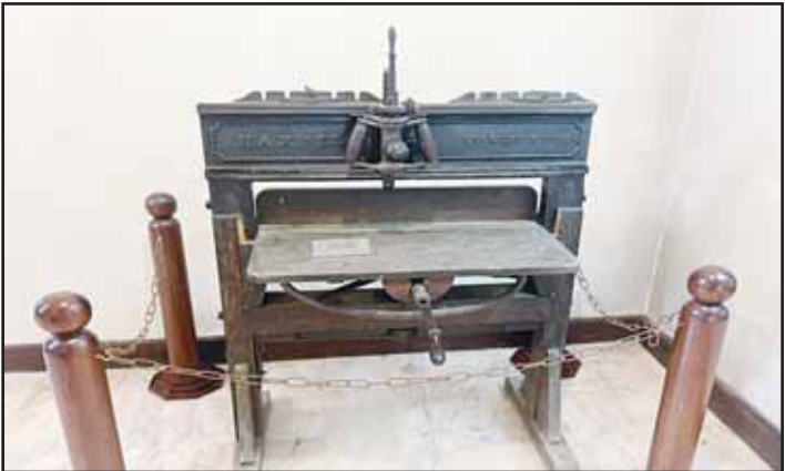
One of the oldest manual printing presses used in the 19th century at the Al-Zakhriya printing press to print pages after arranging the metal letters in the molds.
