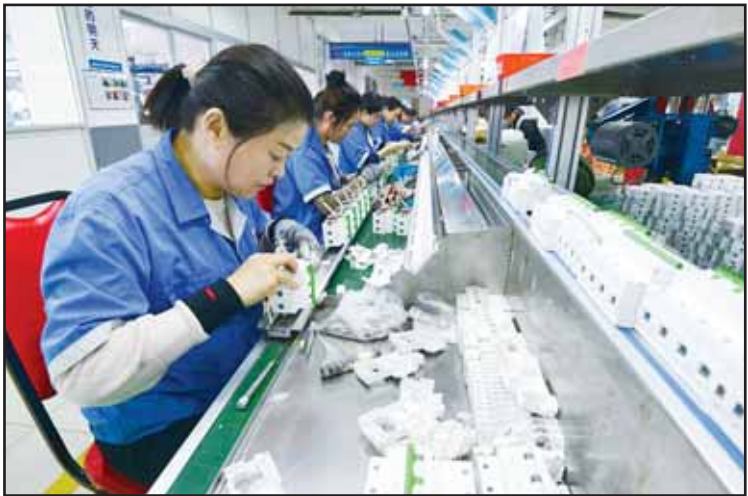
Workers assemble circuit breakers at a manufacturer of electronic equipment, in Fuyang city in central China's Anhui province on April 15, 2025. (AP)
