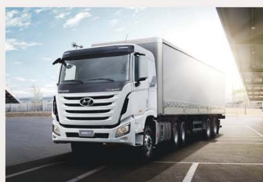
XCIENT Tractor head KD 20,250 MY 2020, 430HP Turbo charge with P.T.O, King Pin Dimension 3.5", G.C.W 70 ton
