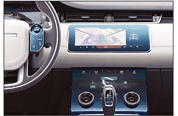
New Range Rover Evoque interior showing its world-first Ground View technology features.
