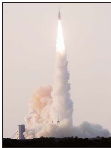
A NASA Orion spacecraft lifts off from pad 46 at the Cape Canaveral Air Force Station on July 2 in Cape Canaveral, Fla. This launch is for a test of the capsule's launch abort system (LAS), which is a rocket-powered tower on top of the crew module built to very quickly get astronauts safely away from their launch vehicle if there is a problem during ascent. (AP)
