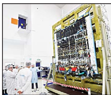
A technician in the cleanroom explains details about the Eutelsat Quantum satellite, billed as the first commercial satellite to be fully configurable in orbit, at Airbus Space and Defence in Portsmouth, southern England on Feb 26. (AFP)
