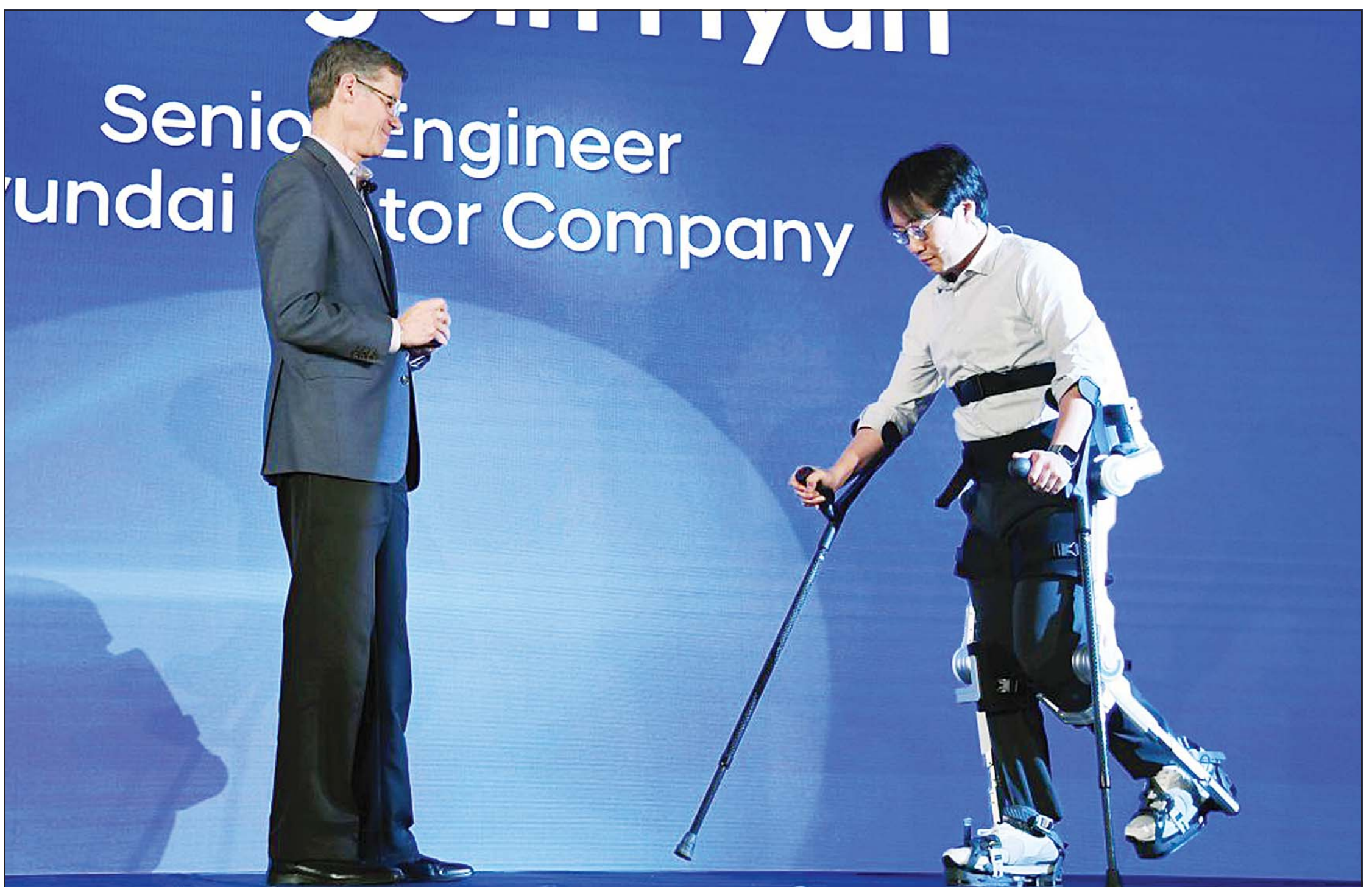
In this file photo, Hyundai Motor Co Vice-President Mike O'Brien (left), looks on as Hyundai Motor Co senior engineer Dr Dong Jin Hyun demonstrates the H-Mex Hyundai Medical Exoskeleton, which is used to assist people who have trouble walking, on Jan 4. (AFP)
